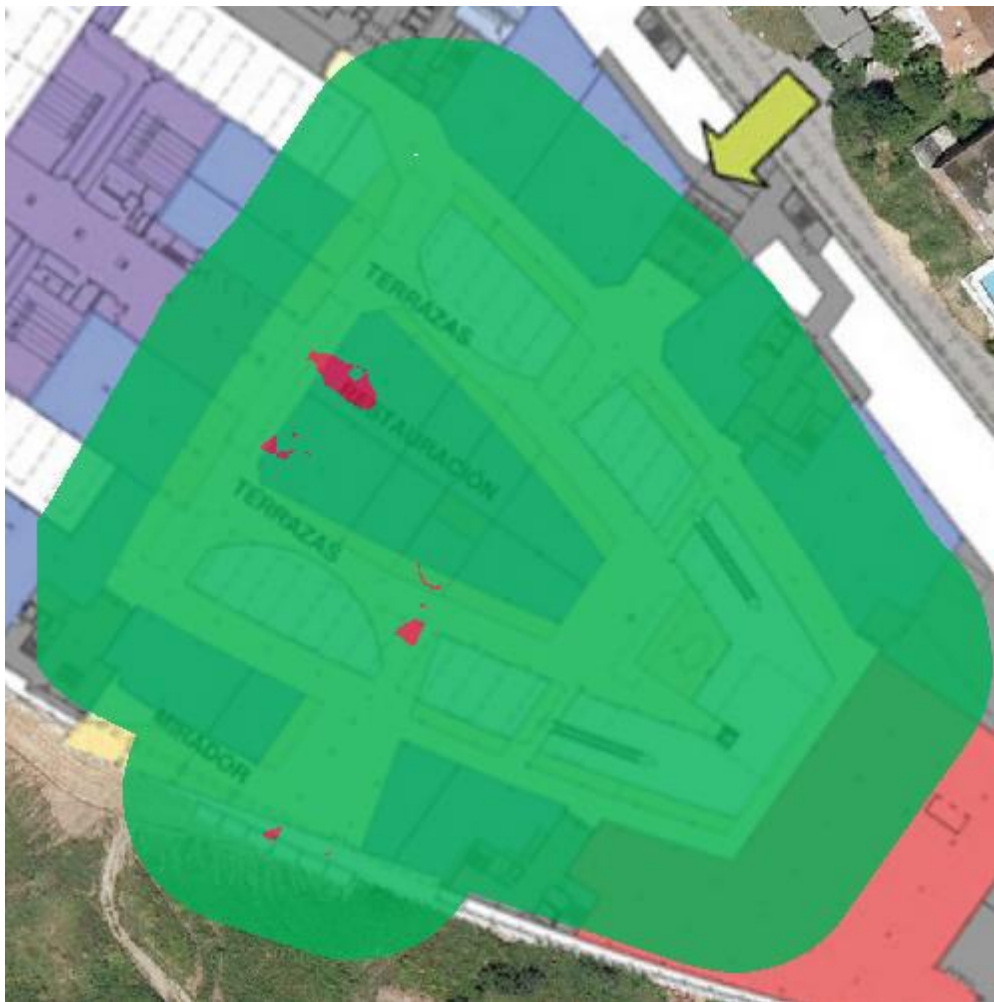
Co-Channel Interference for the network AsCancelas
